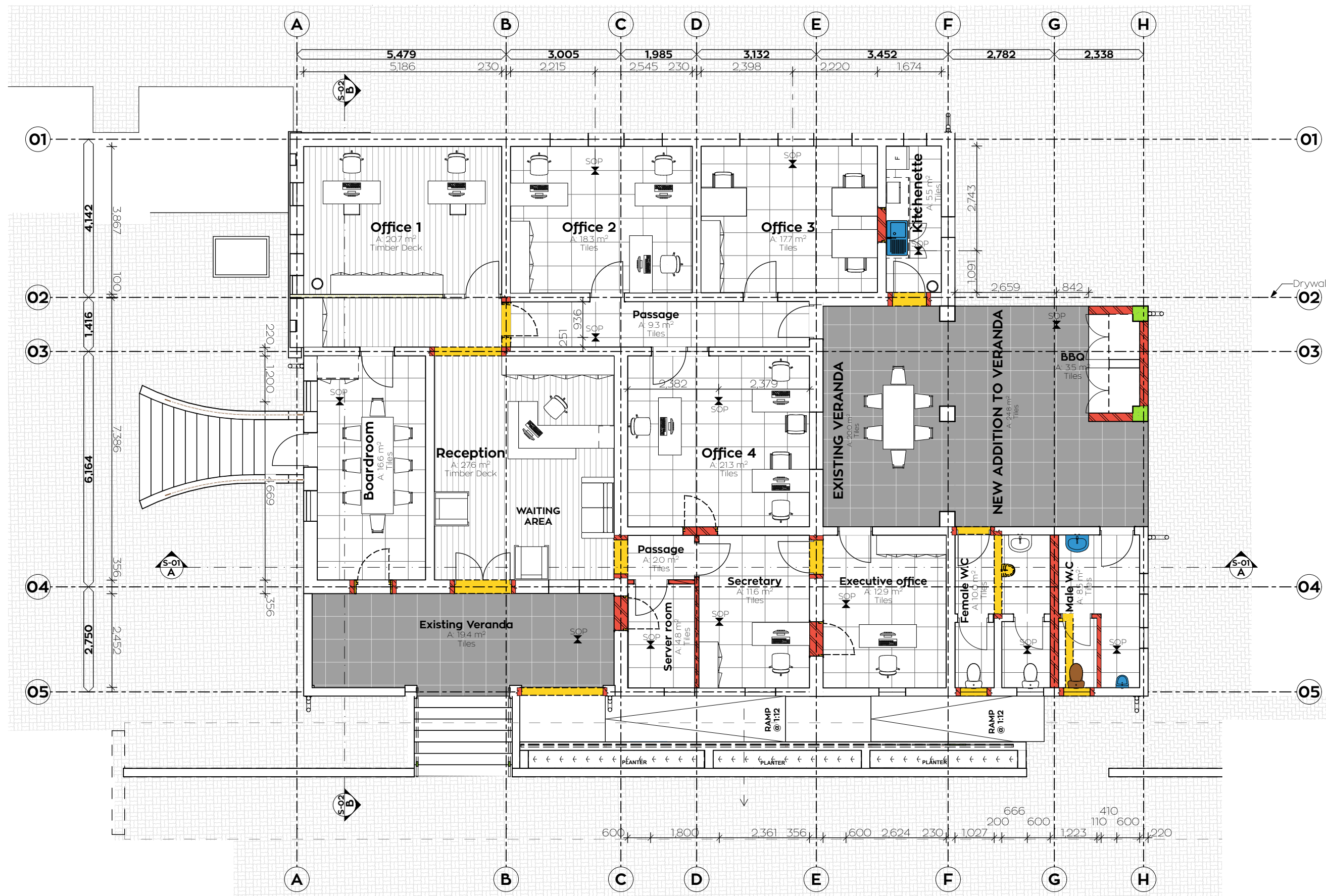
EXISTING BUILDING GROUND FLOOR TILING LAYOUT SCALE 1:100
