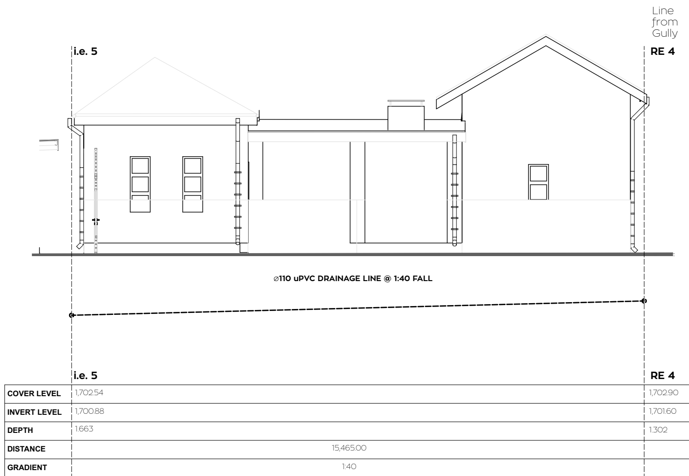
DRAINAGE SECTION 3 SCALE 1:100
