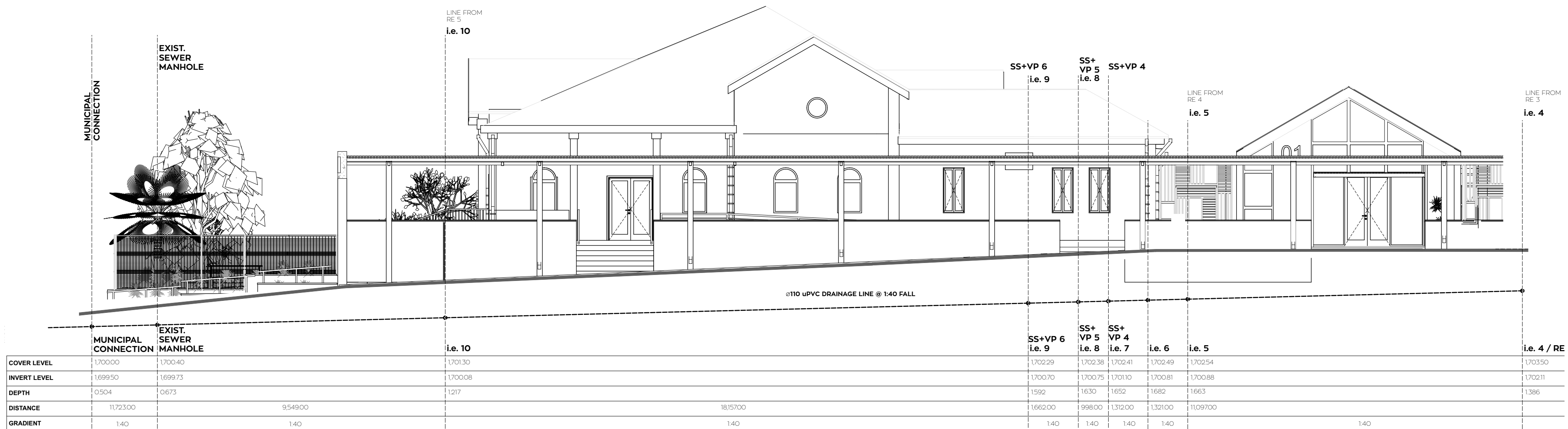
DRAINAGE SECTION 5 SCALE 1:100
